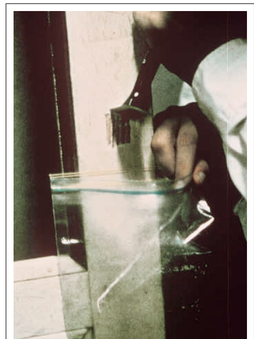
FIGURE 7.5 Removing paint-chip sample.
