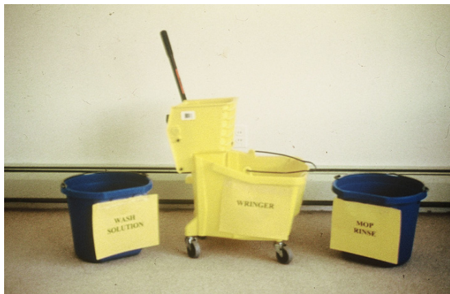
FIGURE 14.4 Three-bucket cleaning system.
