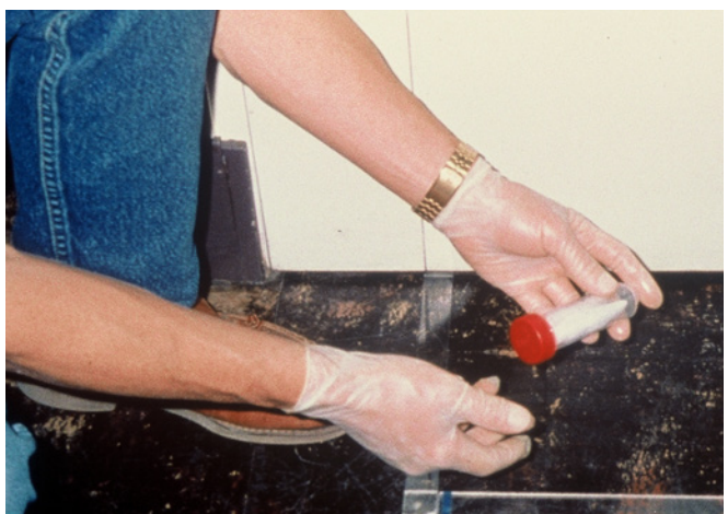
FIGURE 5.11f Placing the wipe into a hard sample container.
