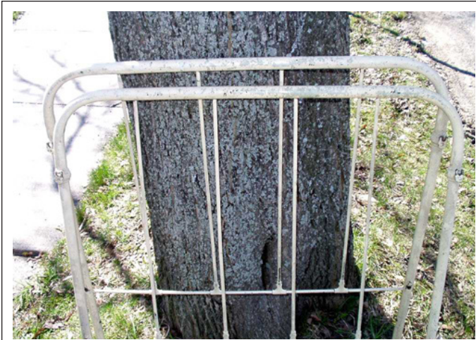
FIGURE 7.2 Child's bed showing teeth marks in the painted surface. Paint should be tested for lead.
