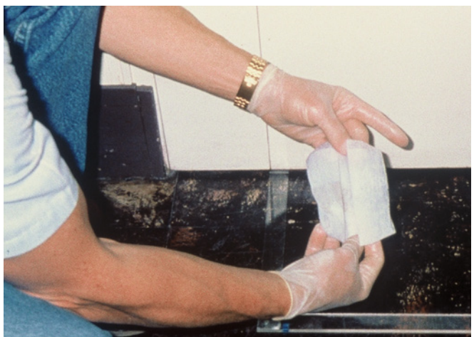
FIGURE 5.11d Folding wipe over for second pass.
